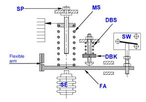
The theoretical articulation axis of the flexible arm "FA" comprises a stainless steel strip that provides constant support for the arm.
