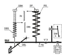
After the set point is exceeded, the movement of the "FB" balance is detected by the switch "SW" used at the end of travel.
